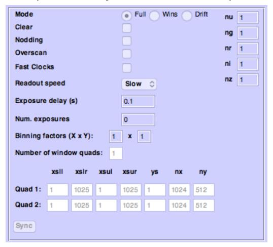
As you make changes to this panel, the displayed FoV will update to reflect your choices of readout mode and window settings. The exposure time, cadence and signal-to-noise estimates in the panel above will also update.
