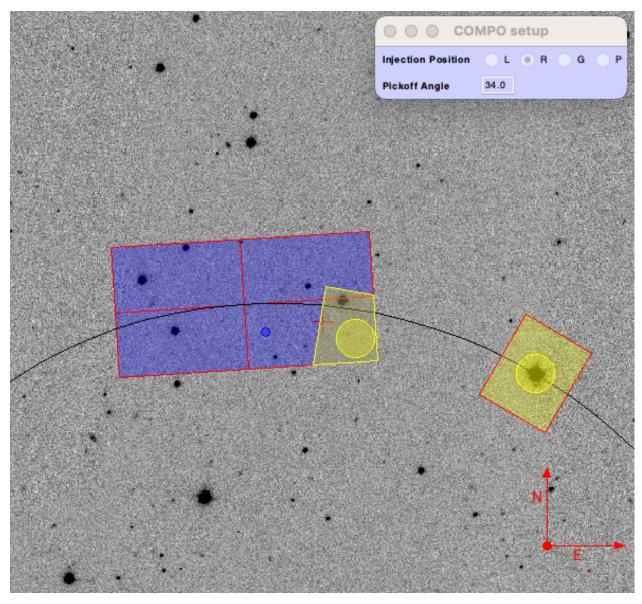
The pickoff and injection arms are shown in yellow. The rectangular region shows the vignetted area, and the circle shows the field of view of the arms. The black line shows the path the pickoff arm will take as it rotates.
